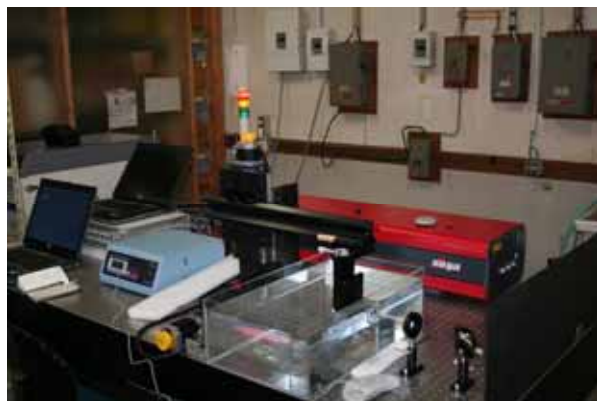
Fig.3 Indirect laser peening system used
