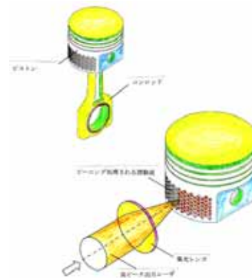
Fig.1 Application of ILP process to piston head
