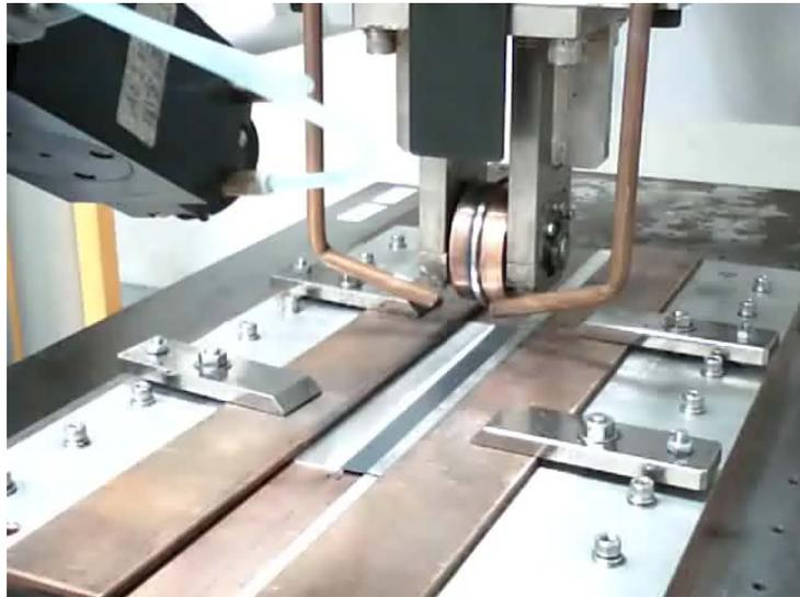
Fig. 5 Laser roll welding facility using a 2kW fiber laser.
