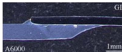
Fig. 18 Macro-section of laser roll welded joint of GI steel to A6000 alloy
