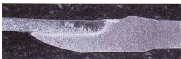
(b) Macro section of overlap butt joint of steel and aluminium alloy
