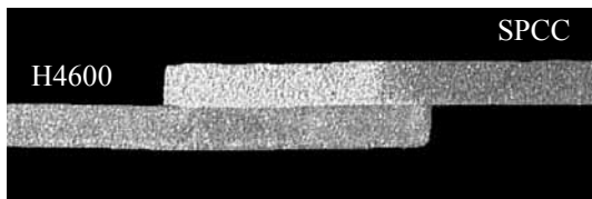
Fig.31 Macro section of SPCC/H4600
