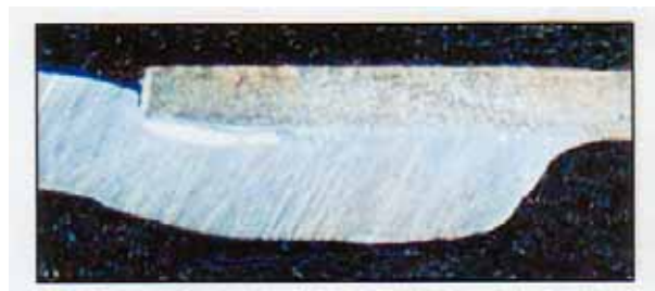
(a) Macro section of overlap joint of steel and aluminium alloy
