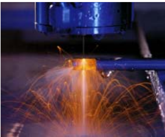
Fig.1 Waterjet-guided laser processing
