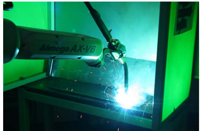
Figure 6 Welding test for contact tip using a robot
