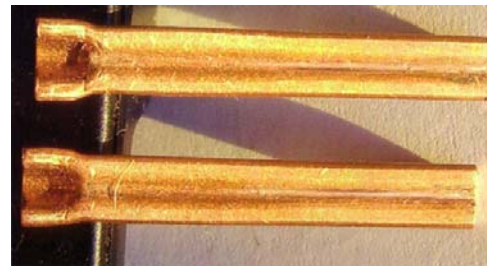
Figure 18 Tip appearance of two piece type contact tip after 50 hours in 8 days in the work shop. (welding current: 120A ~ 160A)
