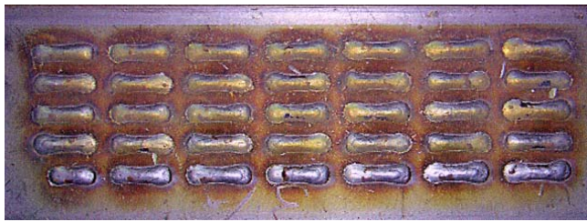
Figure 14 Bead appearance in pulsed MAG Welding using a conventional contact tip.
