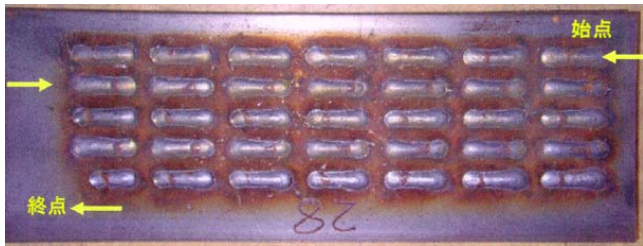
Figure 13 Bead appearance in pulsed MAG Welding using a developed contact tip.
