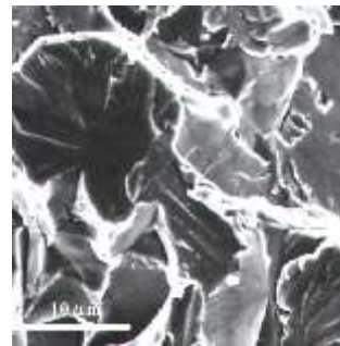
Fig22 SEM image of brittle fracture at clad layer of Colmonoy No5
