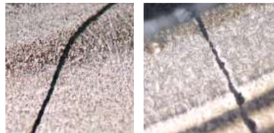
Powder feeding rate 12.67g/min Travel speed 4.5mm/sec a) Colmonoy No5
