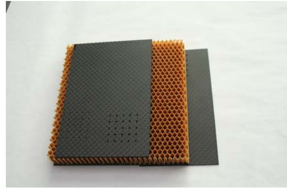
(a) Acoustic liner composed of CFRP and Aramid resin
