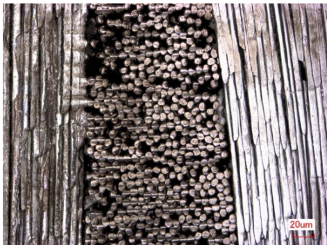
Fig.7 Cross section of thermoplastic CFRP Cut by Q-switch YAG laser
