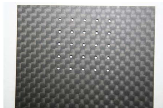
(b) Laser drilling of CFRP panel for acoustic liner (dia. of hole : 1 mm)
