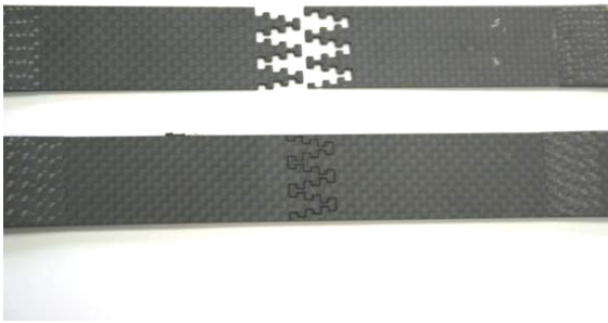
Fig.13 Mosaic Joint of CFRP prepared by laser Ablation
