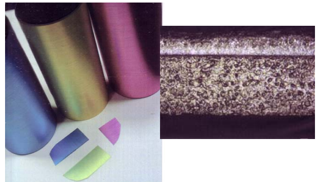
a) polymer—metal composite b) cross section 図4 Laser cutting of polymer-AL—polymer
