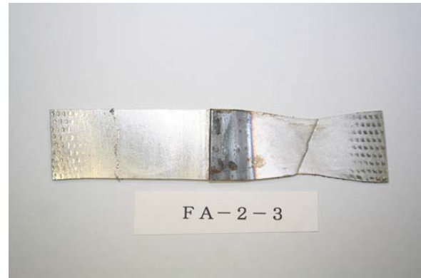
Fig.12 Tensile test specimen of joint FA-2 after test
